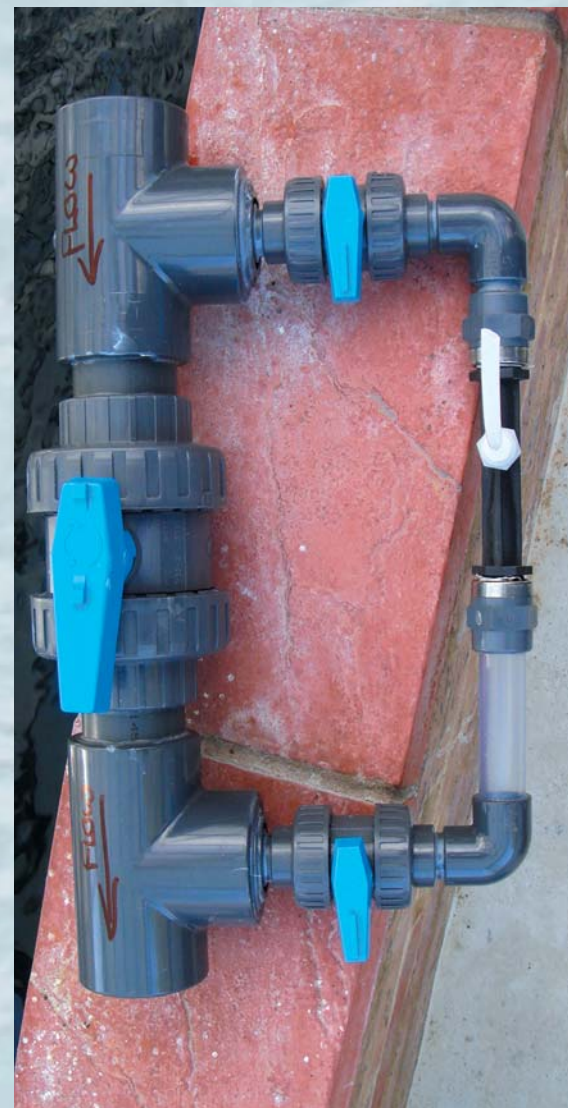
Right: Single venturi injector assembly - for efficient mass transfer of ozone into water feed.
